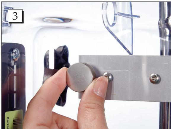
**Step 3.** Tighten the locking wheel on the inside of the pod. Once tightened the POD cannot be removed from the pole without opening the box.
