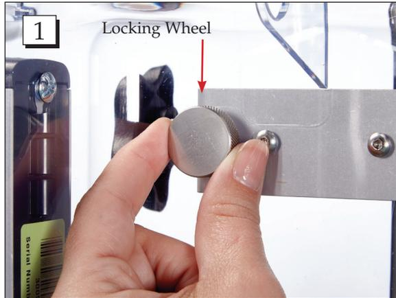
**Step 1.** Open the pod and loosen the locking wheel on the inside of the box.
