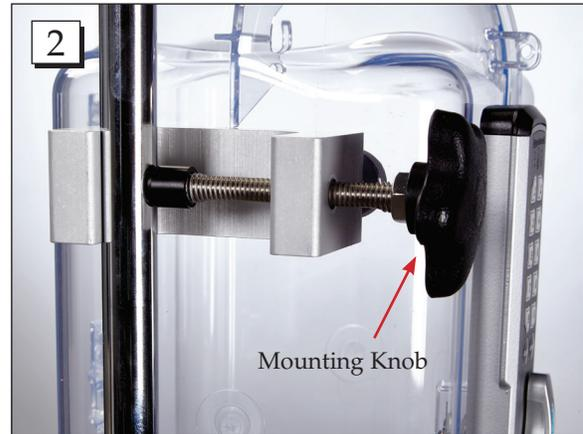
**Step 2.** Turn the mounting knob to make room for the pole. Mount the pod to the IV pole and tighten the mounting knob.
