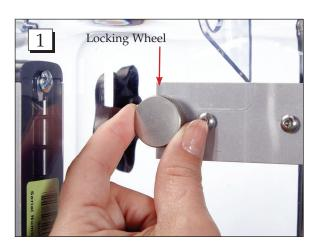
**Step 1.** Open the pod and loosen the locking wheel on the inside of the box.
